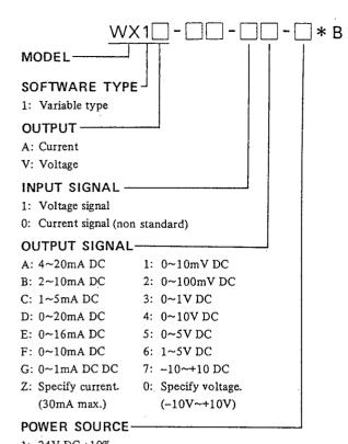
Ordering Information Measuring Range of Input Voltage input signal: 2V min. Span for 0~10V DC Current input signal (input resist:  $250\Omega$ ):  $(250\Omega) \times (Input current)$  shall be within the measuring span of voltage input signal Recommended Range 4~20mA DC 2~10mA DC Current signal 0~20mA DC 0~16mA DC 0~10mA DC 0~10V DC Voltage signal
